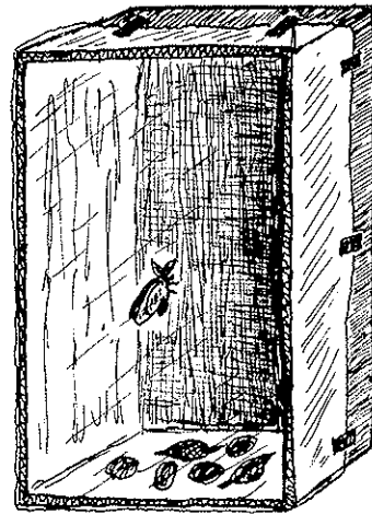
Figure 33. Temporary emergence cage for cocoon-spinning moths. Made from burlap-lined pasteboard box with transparent plastic fastened over the front.
