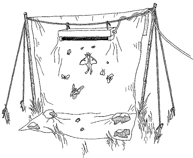
Figure 9. Blacklight set up facing a sheet. Badminton poles were used for support, although wooden stakes would have worked as well.
